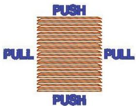
Digitizers must compensate for this movement of the fabric. With experience a digitizer learns how a variety of fabrics will react during embroidery and make adjustments so the design has proper registration.
